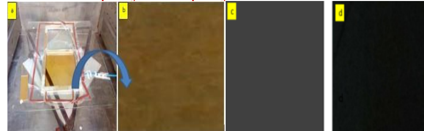
(a) Set up for curing of neat epoxy; (b) Cured neat epoxy sheet (c) Epoxy with 0.1% MWCNTs, (d) Epoxy with 0.2% MWCNTs
