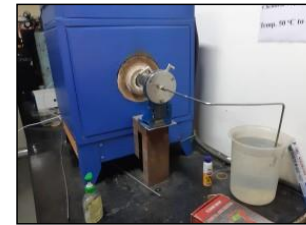
CVD furnace for carbonization
