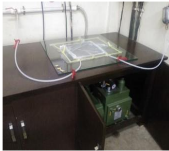
VARTM set up developed in process lab
