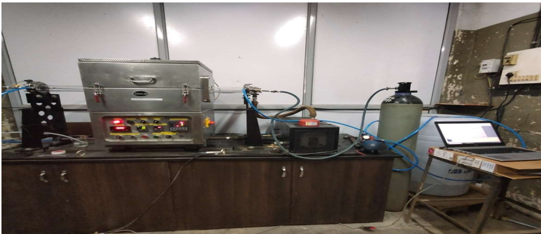
CNT Synthesis using CVD equipment
