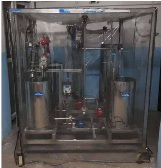
IloT Panel and WaterTreatment Plant Scale down model for ICS-SCADA Cyber Security
